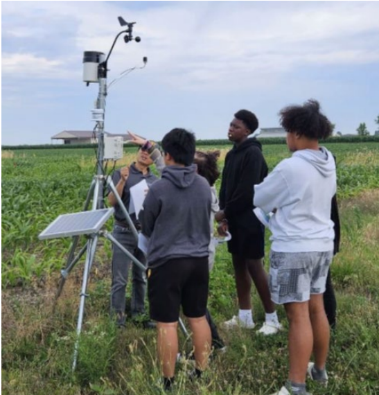
Lincoln University PSI students identify the sensors of a weather station.
